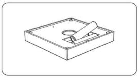
3. Install 2x AAA batteries into the main body of the remote.
