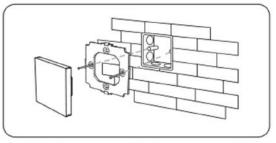
2. Fix the controller base onto the case with a screw.
