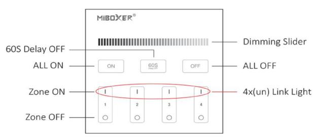
Touch the dimming slider to change brightness from 1% to 100%.
