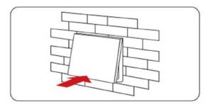
3. Click the upper side of the glass panel onto the controller base, then press the lower slide until you hear it click into place.
